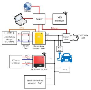
Figure 4: Diagram of the MG charging station for EVs.
