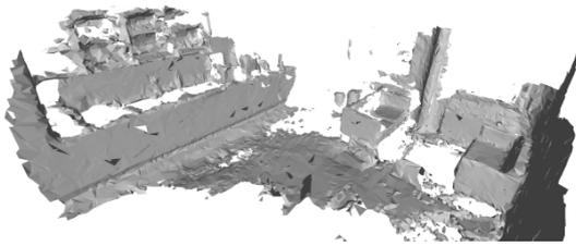
Figure 3: Typical point cloud after scanning a room.
