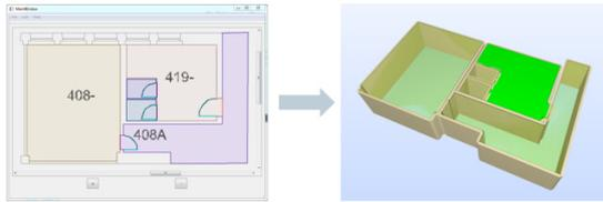
Figure 8: Extrusion of polygons into a 3D model.
