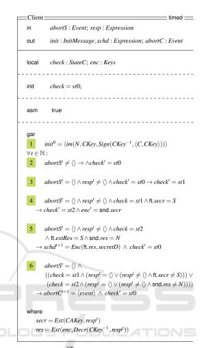
Figure 2: Focus $^{ST}$  specification of the *Client* component.
