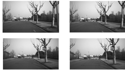
Figure 8: Tracking in Video by Mean Shift. From the upper left to the lower right sub-images represent the 1st, 3rd, 5th and 8th frame respectively.
