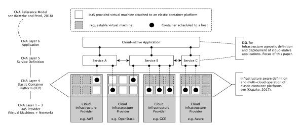
Figure 1: An ECP based CNA deployment for elastic and multi-cloud capable operation.
