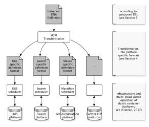
Figure 2: Separation of concerns in deploying a CNA.
