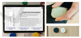
Figure 4: ActiConverge prototype (tablet-based PC with exercise program, Bluetooth beacon, Bluetooth buttons).
