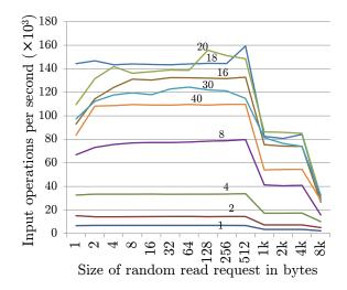
Figure 1: Performance of the tested SSD for 10,000 random reads using different query depths (1 to 40) and for varying sizes of read requests (1 to 8,196 bytes).
