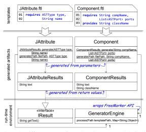
Figure 9: Different cases of template signatures and derived template interfaces.
