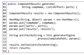
Figure 10: Derived generate() method of the Component interface that returns an instance of ComponentResults.
