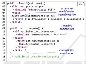
Figure 2: Excerpt of a template transforming component models to Java. To this end, it includes the template Attribute (1. 3) for the creation of Java attributes.
