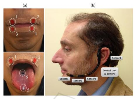
Figure 1: (a) Arrangement of magnetic markers placed on the tongue and lips. (b) Wearable PMA headset with 4 tri-axial magnetic sensors, control unit and battery.
