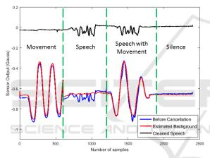
Figure 2: Articulator sensor signal (Sensor3, y-axis) with and without cancellation.
