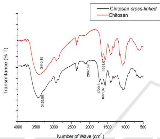
Figure 2: FTIR Spectra of Cross-linked Chitosan and Chitosan Films
