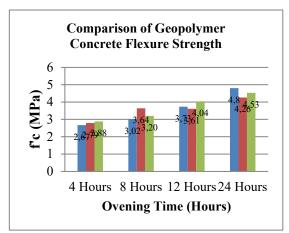
Figure 5: Flexure Strength Comparison
