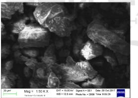
Figure 1: Magnification of Volcanic Ash Samples with SEM Test
