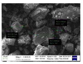
Figure 2: Magnification of Volcanic Ash Samples with SEM Test
