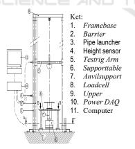
Figure 1: Free fall drop test impact
