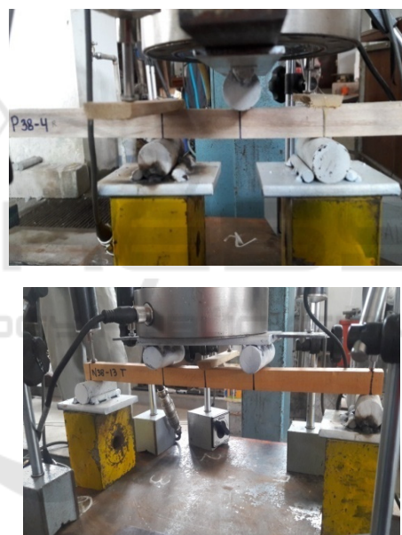
Figure 6: Photos of conducting tests. 3 PB (top). 4 PB (bottom)
