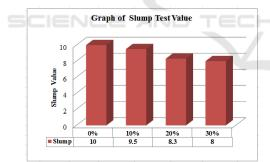
Figure 3: Graph of Slump Test
