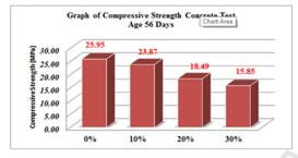
Figure 5: Graph of Compressive Strength Concrete Test Age 56 Days
