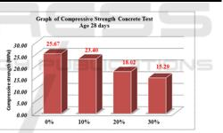
Figure 4: Graph of Compressive Strength Concrete Test Age 28 Days
