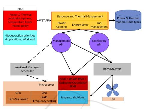
Fig. 7. RTM module architecture.
