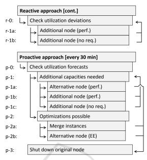
Fig. 5. Illustration of workload allocation algorithm.
