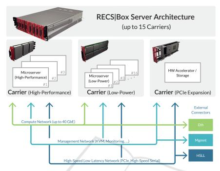
Fig. 1. Overview of the M2DC hardware platform RECS Box.
