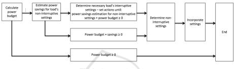
Fig. 6. PCM procedure schema.
