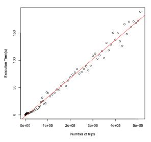
**Fig. 9.** Execution time of PCA and clustering w.r.t. the number of trips. The red line shows the linear regression model, with equation  $Time = 3.490 \cdot 10^{-4} \cdot Size - 2.329$ .
