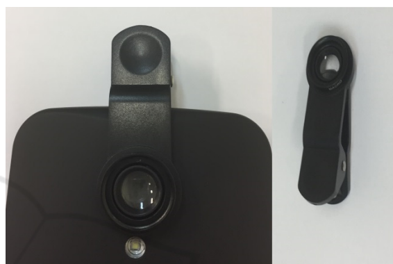
Figure 2: Illustrative image of the macro lens attached to the lens of the smartphone (left) and the macro lens alone with its clipper (right).
