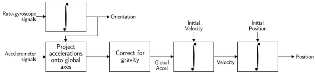
Figure 1: Inertial Navigation System.
