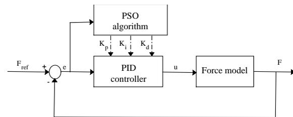
Figure 1: PID controller tuning based on the PSO algorithm for muscular force control.
