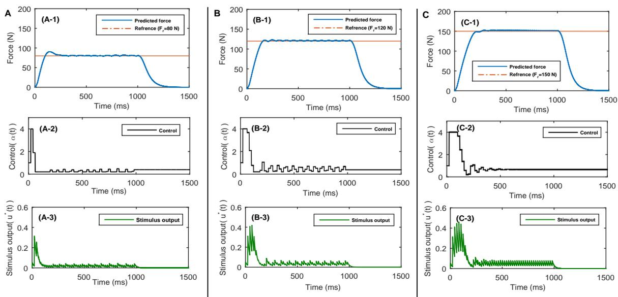
Figure 5: The performance of the PID based PSO control of the muscle force during 1s stimulation session for three desired forces (A:  $F_{ref}=80N$ , B:  $F_{ref}=120N$ , C:  $F_{ref}=150N$ ) using the modified pulse train MCFT30. (A,B,C)-1 illustrate the developed force to track the desired force, (A,B,C)-2 illustrate the computed pulse amplitude  $\alpha(t)$  and (A,B,C)-3 illustrate the corresponding stimulus output applied to the quadriceps muscle.
