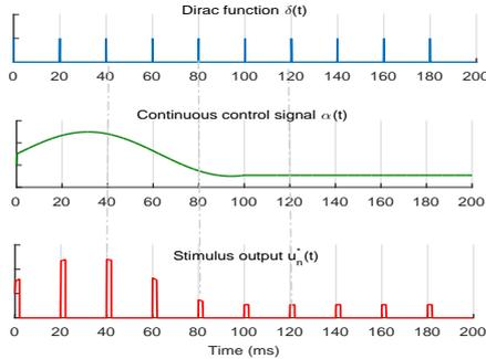
Figure 2: Schematic representation illustrate the proposed method to compute the pulse amplitude on the control of the muscle force by FES systems.
