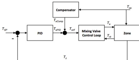
Figure 1: Temperature control scheme.
