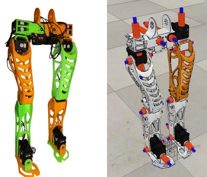
(a) 3D printed prototype. (b) Model in V-REP.
