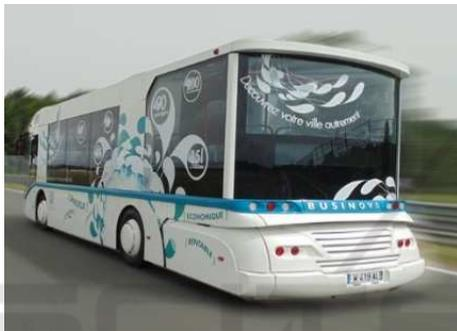
Figure 1: BUSINOVA a Hydraulic-Electric Hybrid bus.
