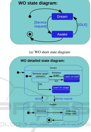
(b) WO detailed state diagram Figure 4: WO state diagram.
