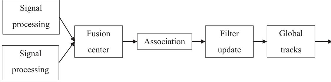
Figure 1: The structure of centralized fusion.
