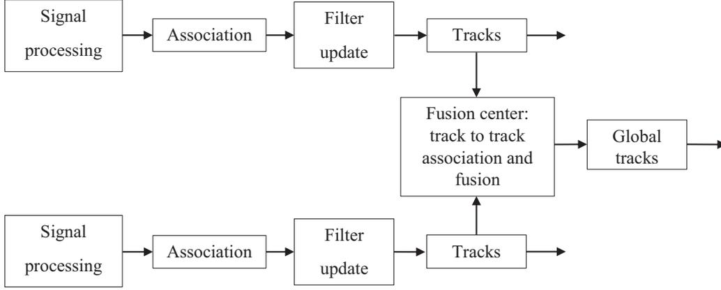
Figure 2: The structure of distributed fusion.
