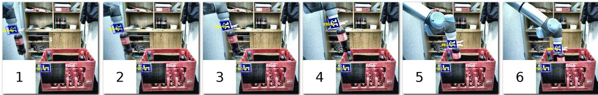
Figure 8: The full action sequence: visual servoing (1-4) and Peg-in-Hole (5-6).
