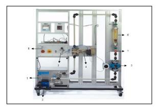
Figure 4: Experiment setup of a flow control (Abraham, 2015).
