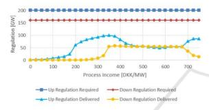
Figure 3: The flexibility potential of the 6 MW ideal process simulations for data from the DK-West Regulating Power Market.
