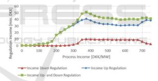
Figure 4: The total regulation income of the 6 MW ideal process simulations for data from the DK-West Regulating Power Market.
