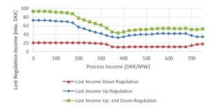
Figure 5: The lost regulation income of the 6 MW ideal process simulations for data from the DK-West Regulating Power Market.
