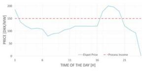
Figure 2: Example of the ON / OFF for the ideal process. The process is ON below the constant line.
