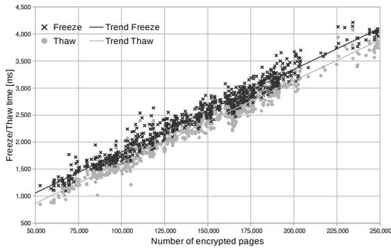
Figure 8: Performance of container freezes (crosses) and thaws (circles) in relation to the number of encrypted pages.
