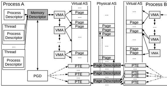
Figure 7: Linux memory management data structures and modifications highlighted in gray colors.
