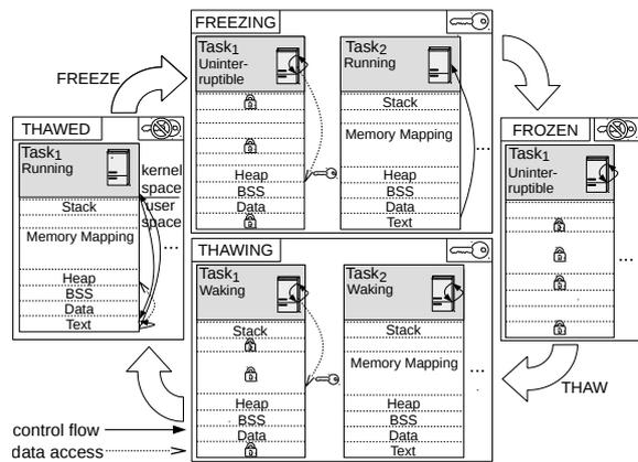
Figure 1: The four states of the freezer along with the behavior of tasks in the different states.
