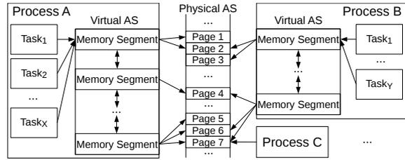
Figure 3: Relationship of processes and threads, their memory mappings and sharing of resources.
