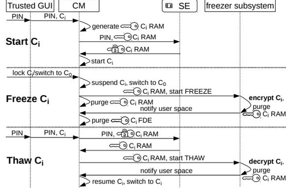
Figure 6: Chronological sequence for starting, freezing and thawing containers along with key management operations.
