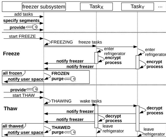
Figure 2: Extensions (bold) to the initialization, freezing and thawing procedures of a cgroup with its tasks in F&C.
