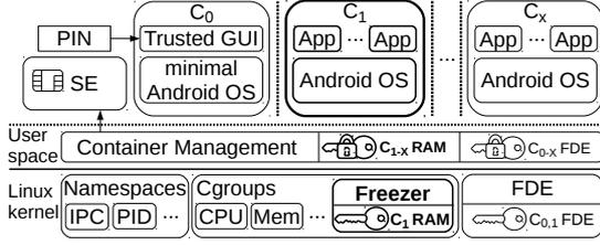
Figure 5: Most relevant components and extension of the virtualization platform for mobile device.
