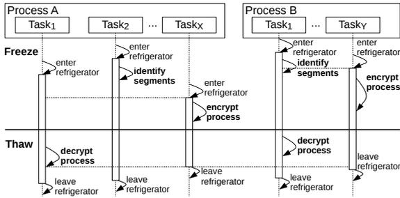
Figure 4: Synchronization of tasks entering and leaving the refrigerator during freeze and thaw.
