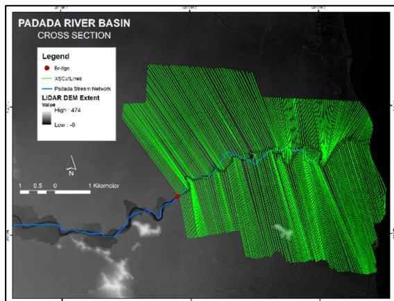
Figure 4: Padada riverbed cross-section data.
