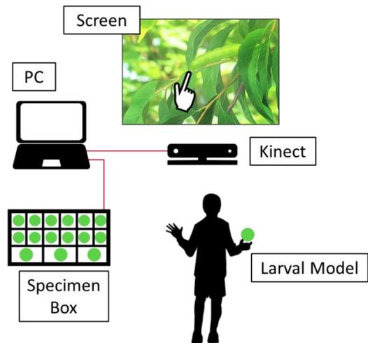
Figure 1: Setup of the system. Function (a) is performed in the specimen box. This consists of Arduino and FSR sensor. Function (b) is performed by the Kinect sensor.
