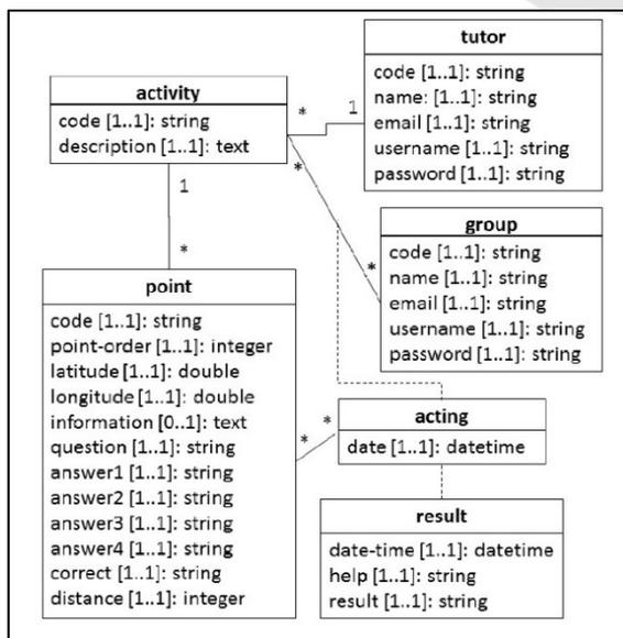
Figure 2: RouteQuizer database UML diagram.
