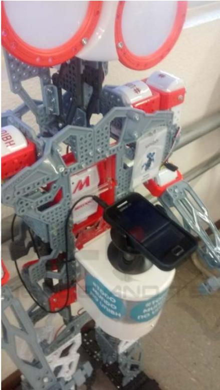
Figure 3: Ozires received an automatic alcohol hand sanitizer dispenser and a cell phone. All lessons given by the robot are produced in the cell phone by using a “change voice app” that produces robotic voices.
