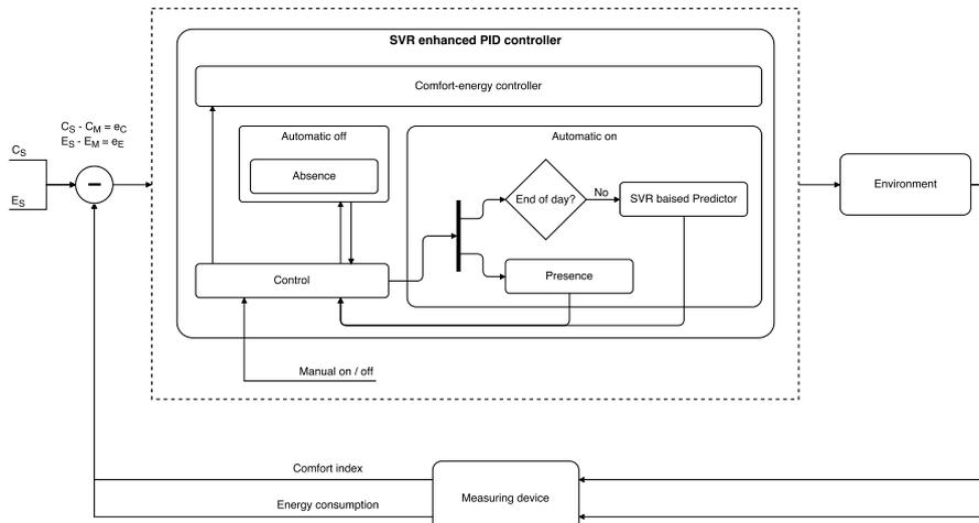
Figure 1: SVReCLCE control loop and its elements.
