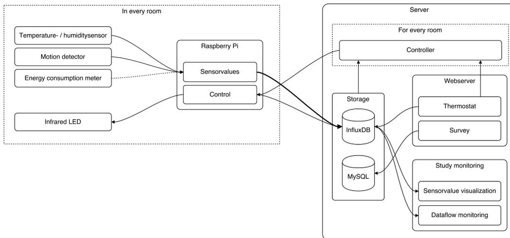
Figure 3: Overview of the HW and SW experimental infrastructure.
