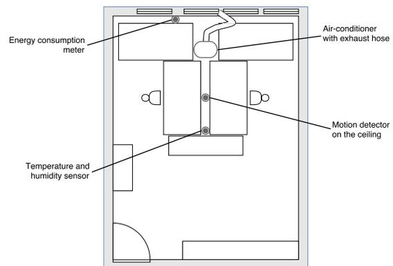
Figure 2: Sensor and actuator deployment.
