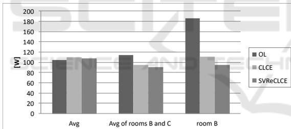
Figure 4: Average Power consumption [W] of our tested controllers among all three rooms (Avg), among rooms B and C and at room B.
