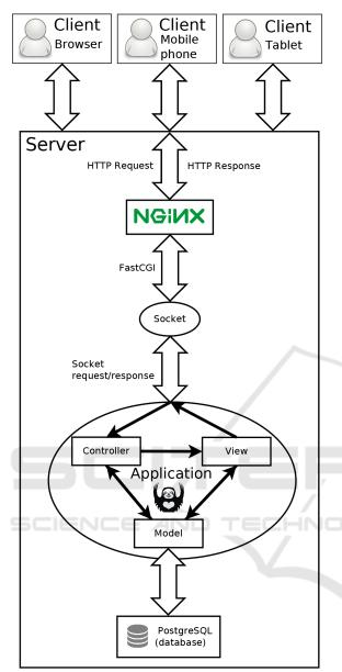
Figure 2: Software prototype architecture.
