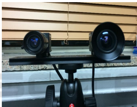
Figure 5: The heterogeneous camera system used in our proposed method. Left camera is the wide field-of-view fish eye lens camera (focal length \cong 3.5 mm). Right camera is the narrow field-of-view conventional camera (focal length \cong 8 mm). Both cameras are mounted on a steel panning bar.
