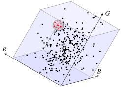
Figure 2: The pixels of current patch are visualized as points in RGB color space. The purple sphere demonstrates the search environment for the density calculation.
