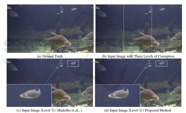
Figure 7: Comparison between the simulated data (level 3) and the results of (Radolko et al., ) (first column) and proposed method (second column). The close up shows the ability of proposed method at preserving the object's detail while eliminating marine snow compared to (Radolko et al., ).
