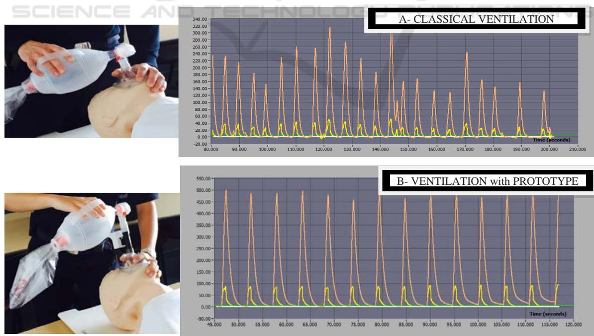
Figure 1: Comparison of ventilation cycle (orange: tidal volume, yellow: airway pressure) without (A) and with (B) our prototype.
