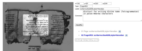
Figure 3: Using the Monk system, the palaeographic expert can select the region of interest (FragmROI), then put the associated attributes (scribe, style, comment etc.) to produce an XML file, which will later be used as labelled data. Currently the experts can only select a rectangular region, but the provision of choosing a polygonal region of interest will be added to the system in near future.
