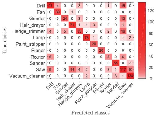
Figure 5: Confusion matrix for identification using  $A_0$  and  $b_3$ . Classification rate CR = 82.98%.
