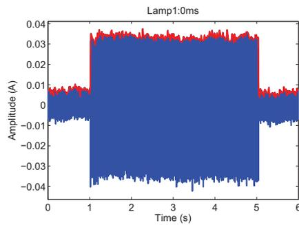
Figure 9: Turn-on transient current of a light emitting diode (LED). The interval  $[0, 1]$  s represents the pre-turn-on period whereas the interval  $[5, 6]$  s represents the post-turn-off period.
