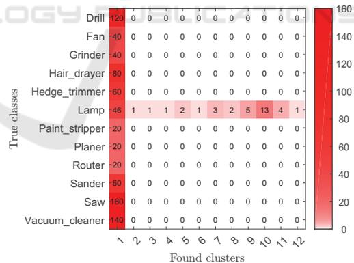
Figure 11: Confusion matrix for clustering using  $A_0$ ,  $b_3$  and  $A_i$ .
