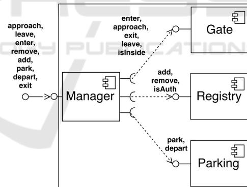
Figure 3: Component model of the initial parking system.
