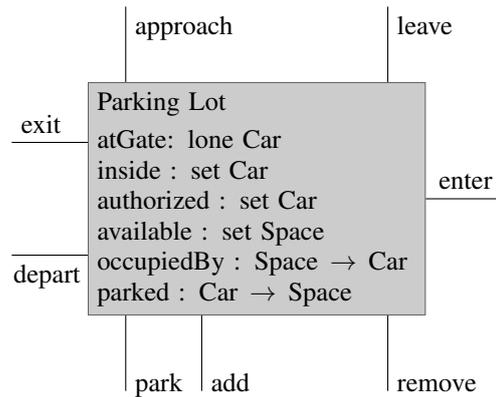
Figure 1: A subsystem diagram that summarizes the entire parking lot system. The system is displayed as a box with its name at the top and the list of state variables inside the box. The system operations appear as line segments emanating from the box, each labeled with the operation name. The keyword *lone* means a set of at most one member.
