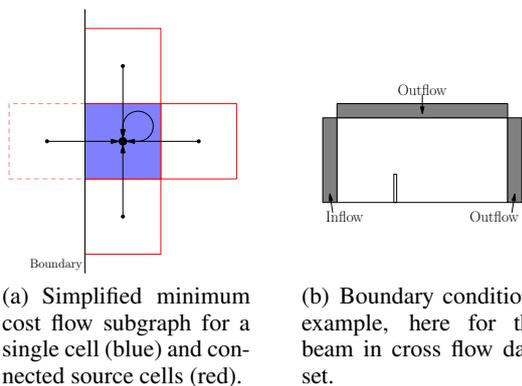
Figure 1: Establishing the minimum cost flow network graph, and how boundaries are considered.
