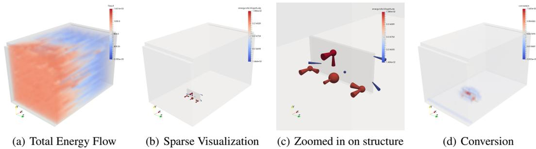
Figure 3: All representations of the energy transport result generated by the minimum cost flow algorithm. (a) The Total Energy Flow clearly shows the decrease of energy along the  $x$ -axis. (b),(c) The Transport Glyph gives a detailed look of a region of interest (the beam) and the surrounding energy flow including the composition of the energy. (d) Finally, the Conversion shows the energy exchange between kinetic and internal energy for the entire domain.
