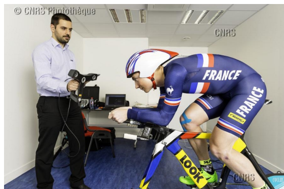
Figure 1: Picture of the 3D scanning setup.
