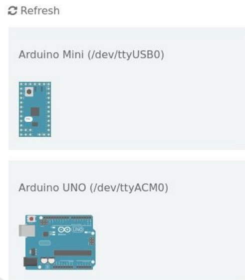
Figure 3: A screenshot of the Remotino tool, showing the two Arduinos which are automatically detected when plugging them into the PC.
