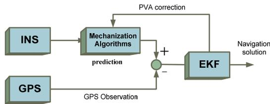
Figure 3: Loose coupling integration scheme (INS/GPS).
