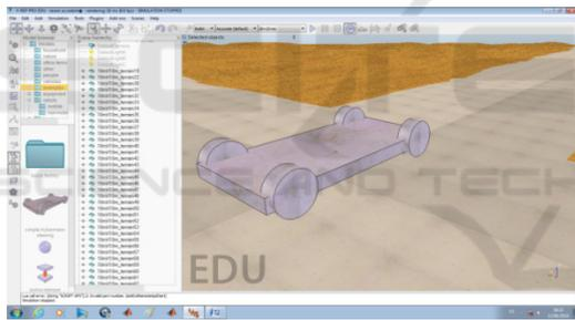
Figure 14: Screen shot of V-REP's application main window.
