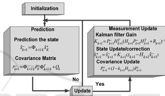
Figure 2: Kalman Filter Algorithm.
