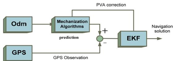
Figure 4: Loose coupling integration scheme (GPS/Odm).
