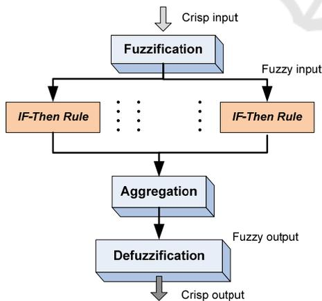
Figure 8: Block diagram of the fuzzy inference system (Wang, 2006).
