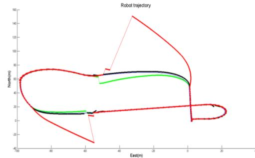
Figure 15: Estimated and reference trajectories: bleu for reference, Red for GPS/INS, Green for GPS/Odm, black for the GPS/RISS integration.
