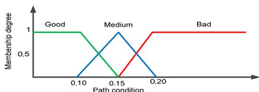
Figure 10 : The first input variable (Path Condition).
