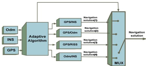
Figure 1: Architecture of proposed integrated GPS/INS/Odm system.
