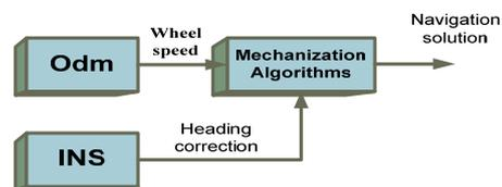
Figure 6: Schematic diagram of the Odm/INS Integration.
