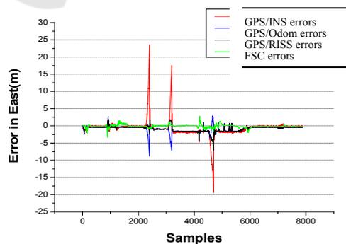
Figure 20: East position Error computed by different integrations.
