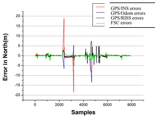
Figure 21: North position error computed by different integrations.
