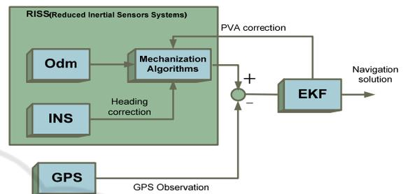
Figure 5: Schematic diagram of the RISS/GPS Integration.
