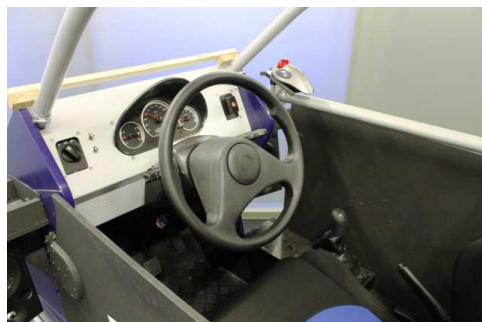
Figure 2: Cabin of the vehicle simulator.
