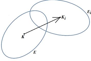
Figure 2: A configuration of a main keypoint  $K$  and its neighbour  $K_i$  for computing *SIFT* descriptor of the latter.
