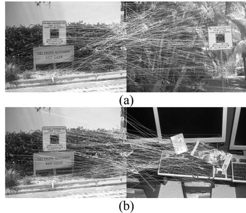
Figure 1: Exemplary matches between affine-invariant keypoints (using SIFT descriptors): (a) for a pair of images sharing a similar object and (b) for a pair of image without similar objects.
