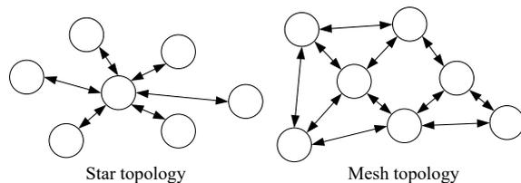
Figure 1: Typical topologies in industrial environments.
