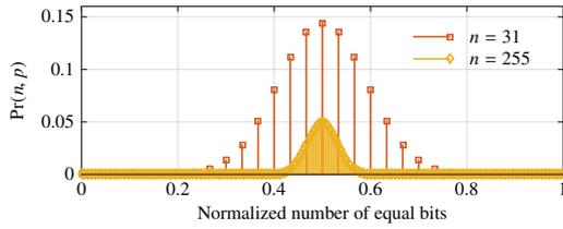
Figure 5: Distribution of equal data bits in  $\mathbf{d}$ .
