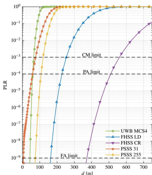
Figure 9: Packet loss rate versus coverage range.
