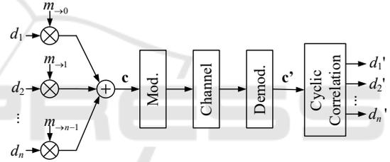
Figure 3: PSSS coding and decoding process.
