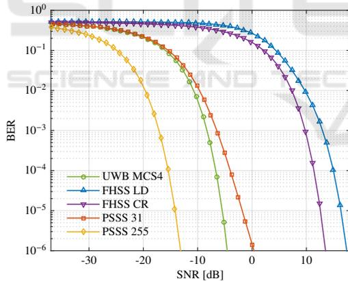
Figure 7: Bit error rate versus SNR.
