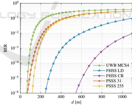
Figure 8: Bit error rate versus coverage range.
