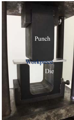
Figure 2: The punch and die components for experiments.
