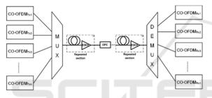
Figure 1: Configuration of Long-distance CO-OFDM transmission system employing midway OPC.
