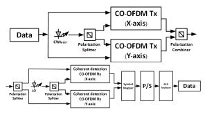
Figure 6: Conceptual diagram for PDM-CO-OFDM system.
