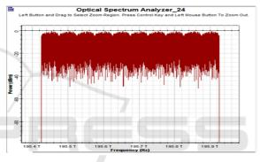
Figure 7: The optical spectrum for 10 WDM CO-OFDM channels.
