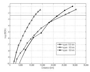
Figure 10: Maximum reach of 10-WDM channels PDM-CO-OFDM 4-QAM systems at 100 Gb/s per channel for each amplifier spacing.
