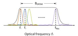
Figure 3: The zoomed-in optical spectrum for one WDM channel.
