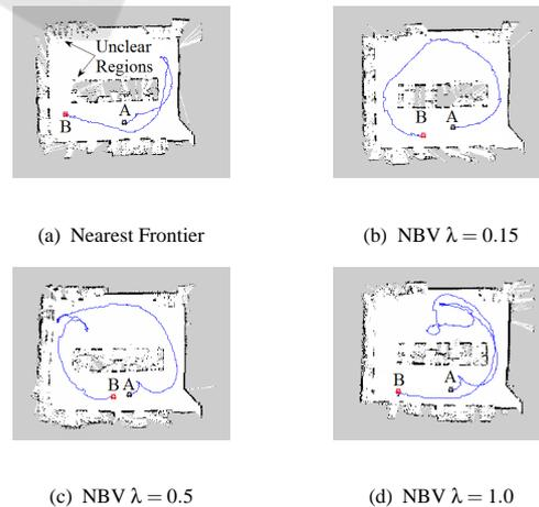
Figure 6: Sample map results for each approach showing the robot trajectory. 'A' and 'B' indicate the initial and final robot poses respectively.
