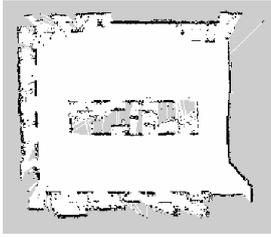
Figure 4: Ground truth map obtained by manually steering the robot in the laboratory environment.
