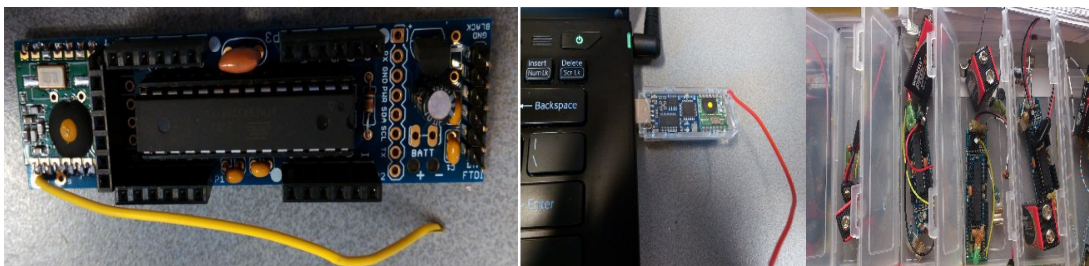
Figure 3: The GSR measuring system: (left) the front side of the sensor board; (middle) the sink node connected with a laptop; (right) the complete sensor sets.
